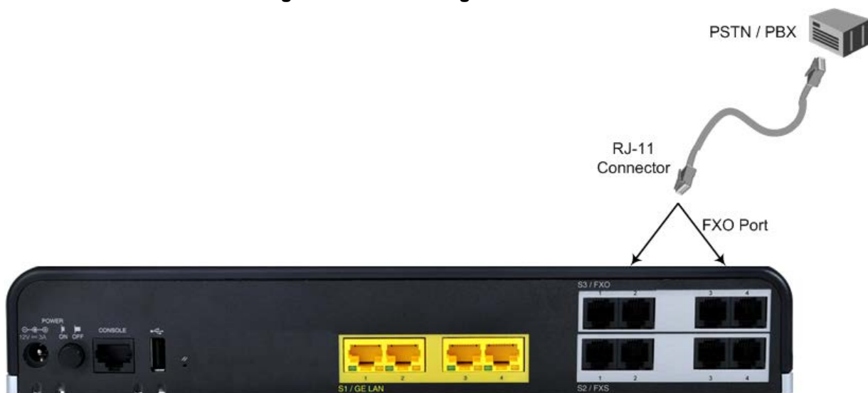
Figure 5-9: Connecting FXO Interfaces
